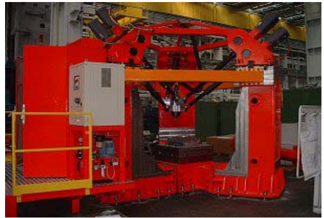
PKM Celerius Designed and developed by ITIA-CNR for the National Programme for Research Into Innovative Production Systems
